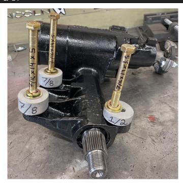
**1961-64 Models Only:** These models will require an upgrade to the 1965-69 model steering box which is smaller and allows clearance to the headers. A steering box retrofit kit is Included with the 1961-64 option.
