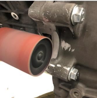
By holding the driver side header in place, it can be seen that the inside tube contacts the engine block and transmission bellhousing. This area should be sanded as shown using a drum sander or similar tool.
