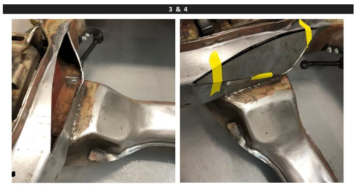
Picture 3 shows the shape that should be removed with a cut-off wheel or similar. It is advised to make multiple trims until the patch part fits as shown. The patch part can be taped into place so that the engine can be installed and clearance verified before any welding is done.
