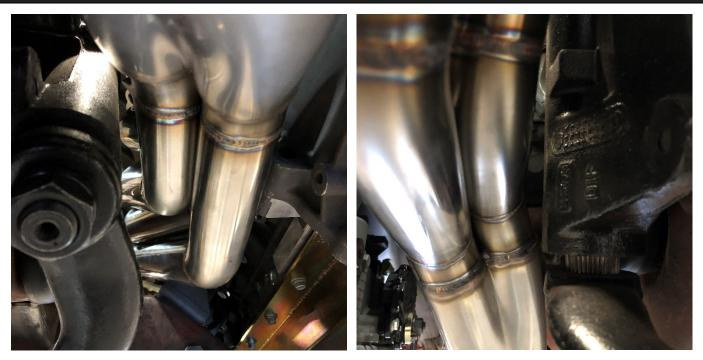
With the engine in place, it is advised to confirm the space between the header and the steering box which should be a minimum of ¼ inch to ½ inch clearance in all places.
