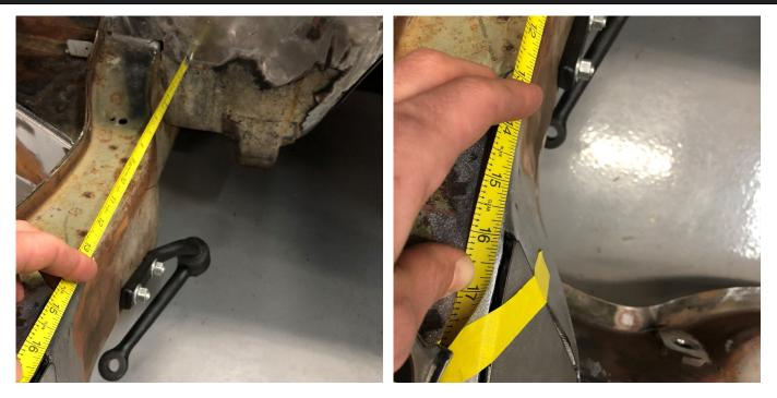
A small patch is required on the passenger side to install the headers. Measuring from the firewall, the back corner of the included patch plate will fit at 16 inches.
