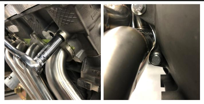
The header can now be temporarily secured and checked to confirm there is space between the innermost tube and the engine and transmission.
